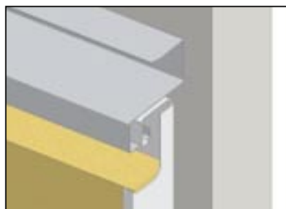
B - B Panel hanging in perimeter profile
